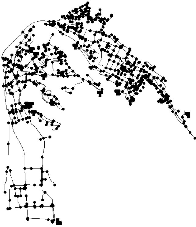
Fig. 1. Haifa-B full model (867 nodes, 987 pipes)
