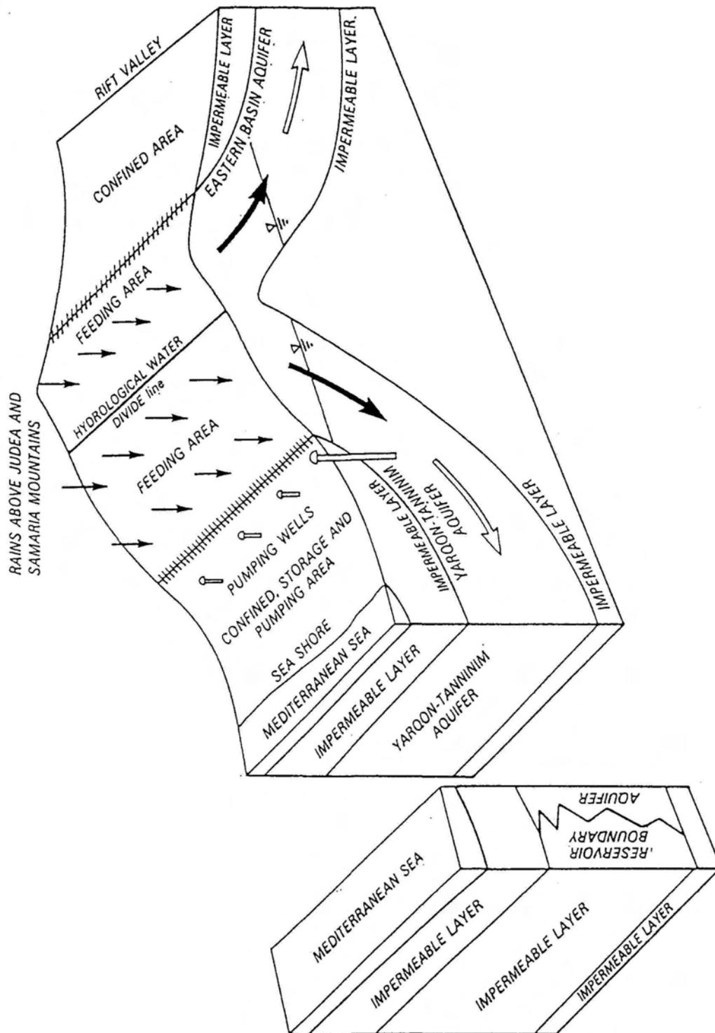
Figure 2. Block diagram of the Mountain Aquifer
